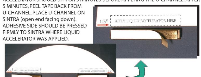
\*LIQUID ACCELERATOR SHOULD SIT FOR 5 MINUTES BEFORE ADHERING U-CHANNEL TO SINTRA. NOTE: USE (1) BOTTLE OF LIQUID ACCELERATOR PER (4) HEADER KITS
